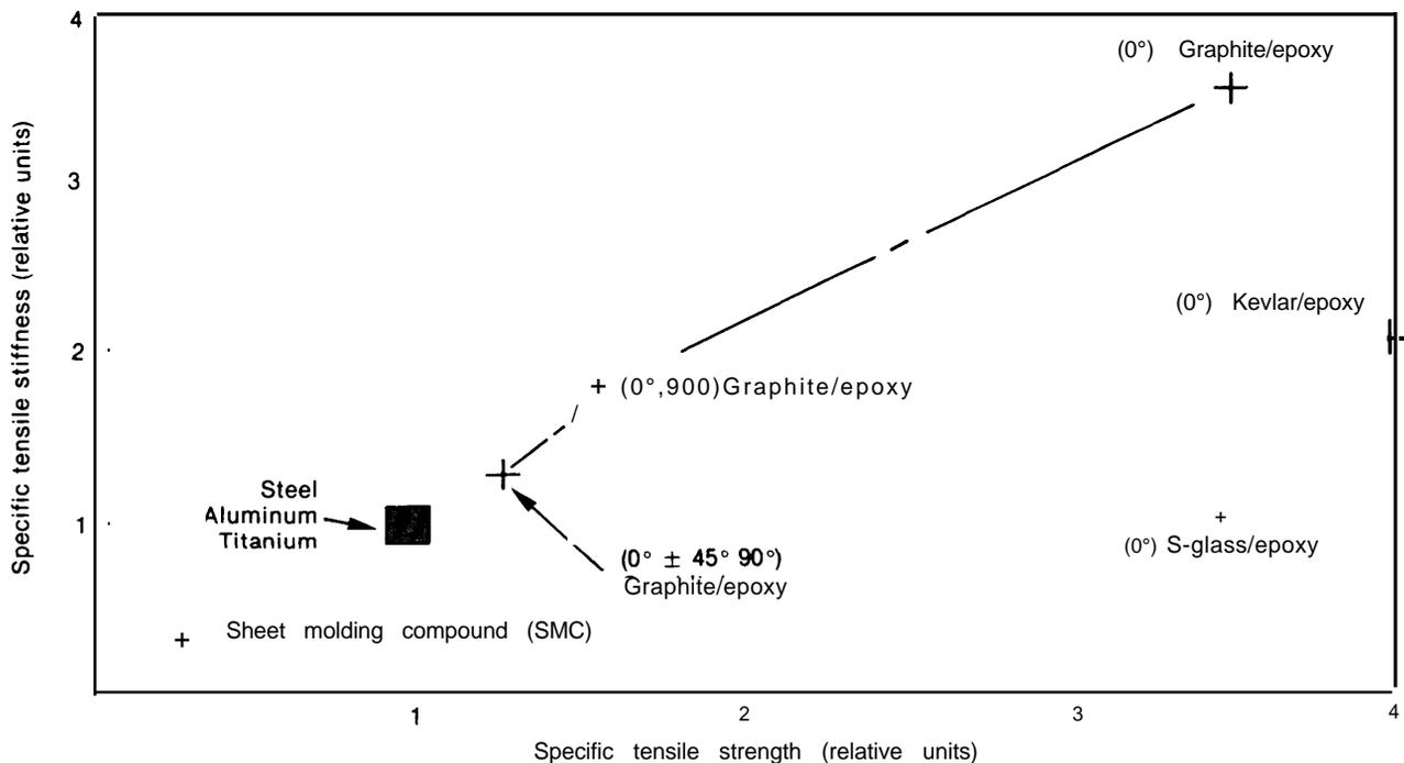
Specific properties are ordinary properties divided by density; angles refer to the directions of fiber reinforcement
